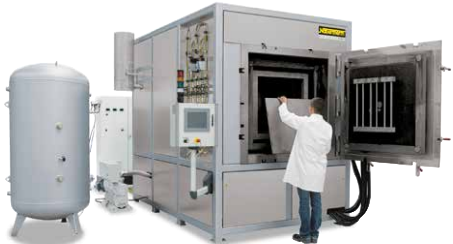
VHT 500/22-GR H 2 with graphite insulation and heating see page 16
