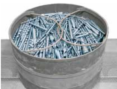
Blueing of drills in water steam atmosphere in a furnace of the NRA range see page 14
