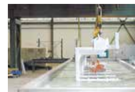
Water quench tank with powerful water-circulation
